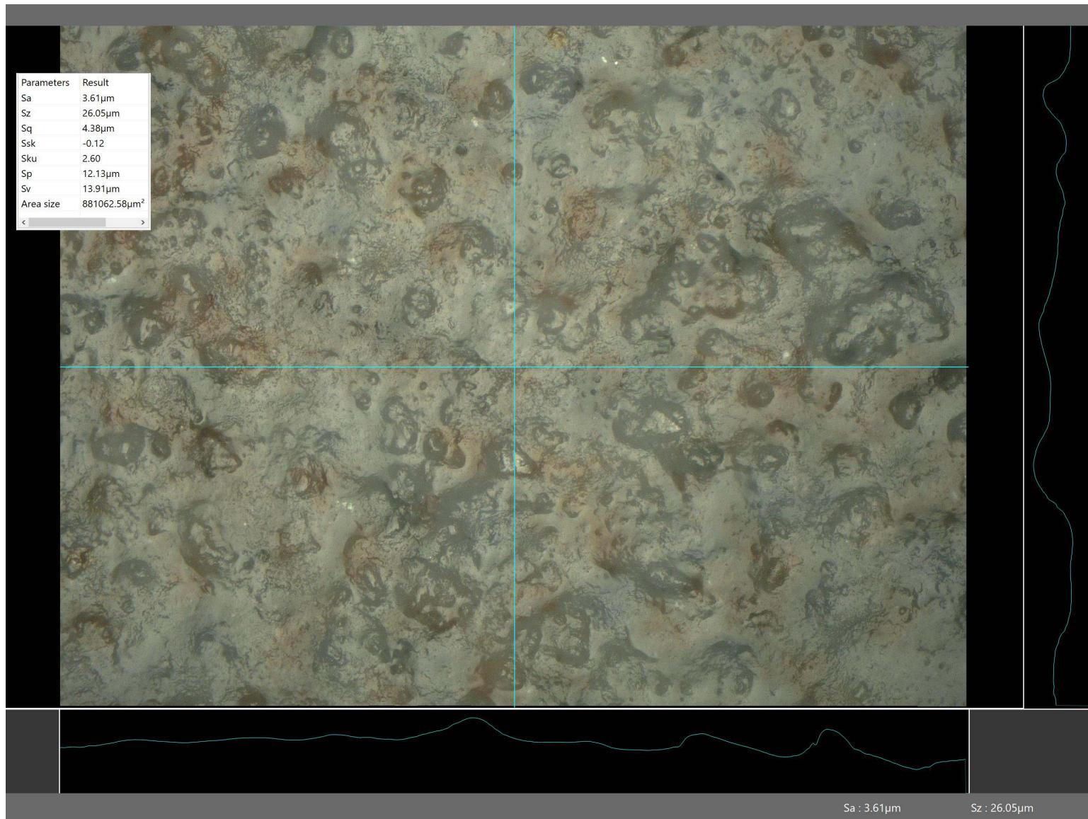
Figure 15. This coaxially illuminated third area of the Good floor tile has the much lower surface roughness parameters given in the embedded table.
