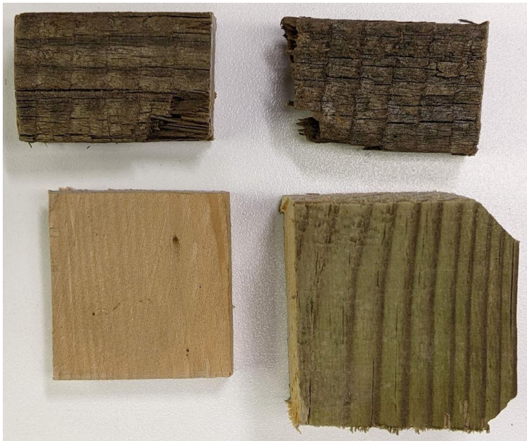
Figure 1. The disintegrating wood received from the surfaces of the bridge wood.
