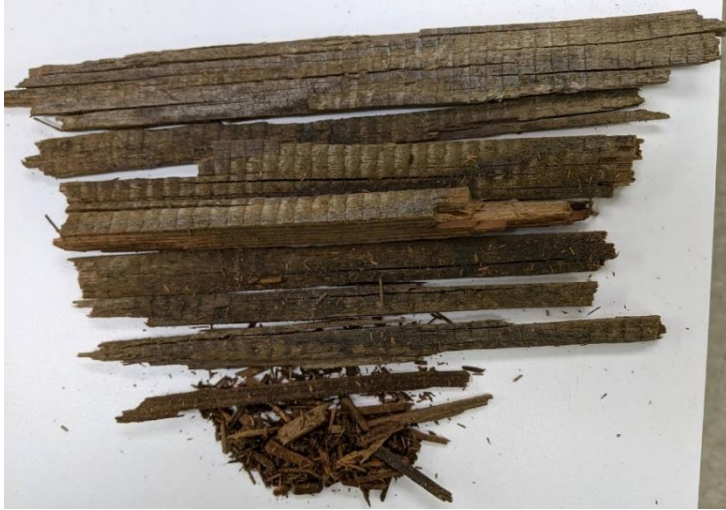
Figure 1. The disintegrating wood received from the surfaces of the bridge wood.
